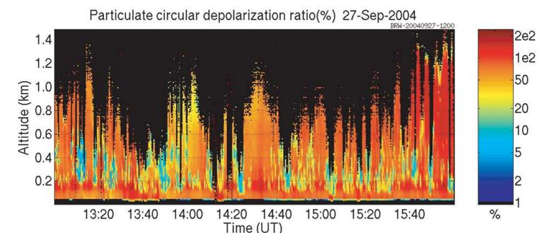
The circular depolarization measured between 13:00 and 16:00 on Sept 27. High depolarizations (red) indicate scattering from ice crystals while low depolarizations (blue) indicate that the optical scattering is dominated by scattering from spherical water droplets. Note that the minimum range observed by the radar is 200 m, thus it is not possible to make the flux computation below the water.
