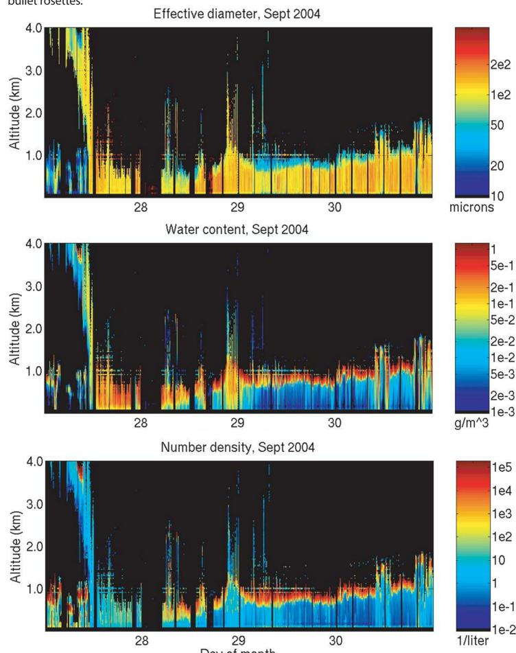
The vertical flux of water can be computed using the radar measured vertical velocity and the lidar-radar derived water content. The flux of water computed an altitude of 250 m using several crystal type assumptions is compared with surface measurements of precipitation in the next figure.
