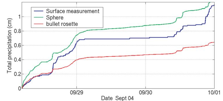
When the surface measurement of the accumulated precipitation (blue) is compared to the lidar-radar derived fluxes after 5:00 UT on 28-Sept, the measurement falls between the results derived for bullet rosettes and spheres. During this period, low level water clouds were not present in 250 m lidar and radar data used for the flux computations.
