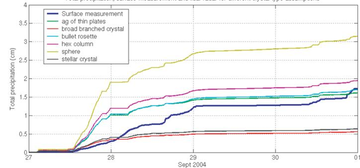
The surface measurement (blue) shows a slower accumulation rate than all of the model results on Sept 27. An examination of the lidar depolarization data for this period shows that water clouds embedded in the snowfall increase the water content at 250 m. It appears that the over prediction of the precip rate results because the radar velocity is highly weighted towards the falling snow and thus the flux is computed assuming that the cloud water is falling at the same velocity as the snow.
