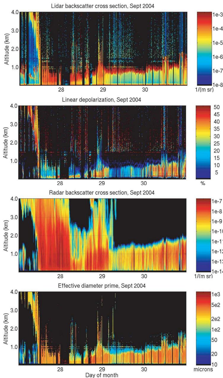
Conversion of 'effective diameter prime' to 'effective diameter' and derivation of water content or number density requires use of an assumed particle size distribution for water clouds and both an assumed size distribution and a crystal type for ice clouds. The following assume gamma distribution parameters  $\alpha=2, \gamma=1$  for water and  $\alpha=1, \gamma=1$  for ice. Ice crystals are assumed to be bullet rosettes.
