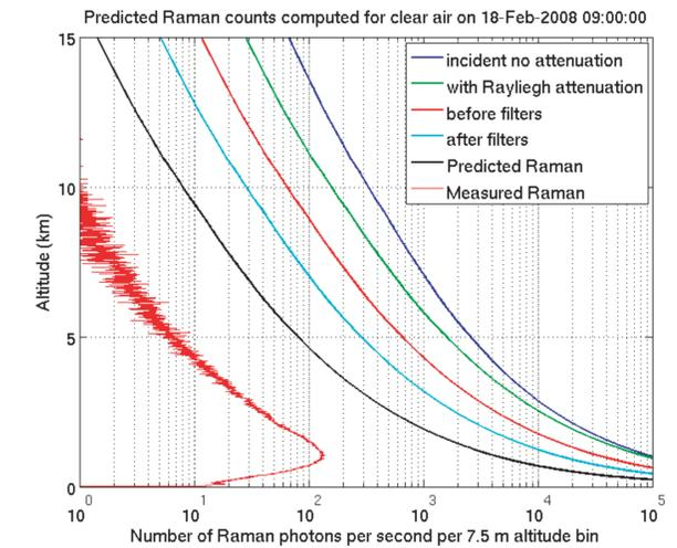
Model predictions of the nitrogen Raman signal compared to an observed profile derived from a 10 s average. The observed profile is an order of magnitude smaller than predicted. The cause is not known. However, differences between the specified and actual optical efficiencies of individual elements are suspected.
