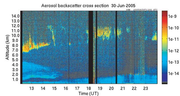
AHSRL observed backscatter cross section in the case used for background noise comparisons.
