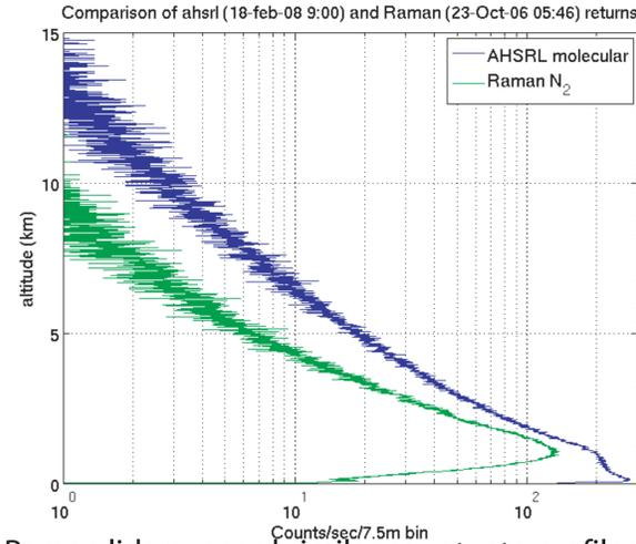
The AHSRL and the Raman lidars record similar count rate profiles. However, both are lower than predicted. Both profiles were computed from 10 second averages of nighttime data with a range resolution of 7.5m. Increased molecular attenuation at 355nm is evident in the faster decrease of the Raman profile with altitude.
