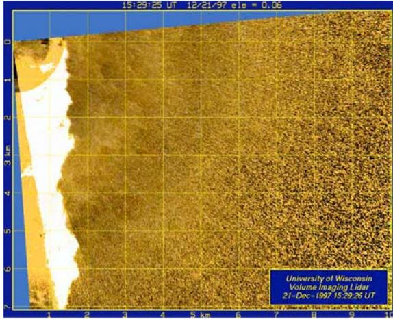
Figure 6: A PPI image enhanced using a high pass filter in order to observe structures in the onshore flow.
