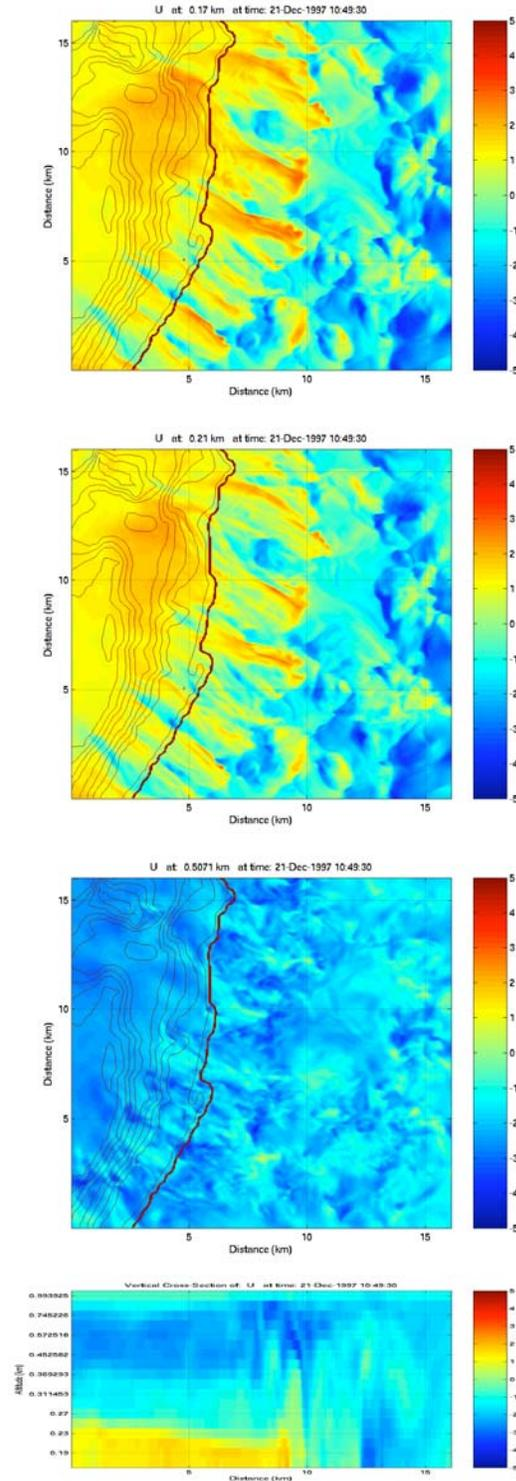
Figure 7: 6<sup>th</sup> grid model output of the zonal component of the flow velocity. The bottom image is a west (left) east (right) cross-section, while the top images are horizontal cross sections at the surface, 40 m, and 330 m, with topography contoured.
